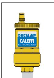
The installation of the valve in places subject to freezing is not recommended. In the case of installation in locations that cannot be inspected, it is recommended to replace the upper caps with the safety hygroscopic caps, code 59681. To allow for the venting of the air during normal operation, the upper cap must be loose (tight in the hygroscopic version).
