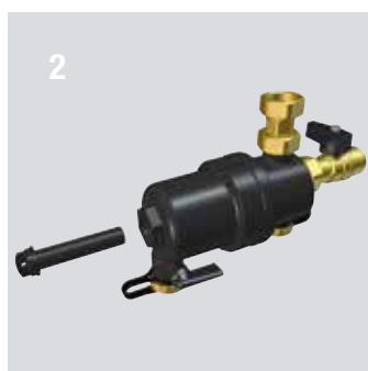
Removing the magnet (turn it 90° clockwise)
