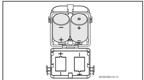
Fig. 4 Colocar as baterias
