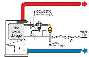
*Installation of the temperature safety relief valve in the emergency heat exchanger.*
