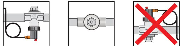
Depending on the fuel stoking system and the open or closed expansion vessel, the sensor of the temperature safety relief valve should be installed on board the machine (with the pocket immersed into the heating medium) or on the flow pipe before any shut-off device (as close as possible to the generator or within the distance where specified by the applicable standard).
