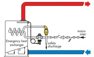
The valve should be installed only on horizontal pipe, with the obturator axis in vertical position. It is allowed the installation of the valve laying on the side (with the obturator axis in horizontal position) but never upside down.
