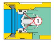
In the event of strong counter pressure, the obturator (2) alters the shape of the seal and rests on the actual end point. This solution guarantees optimal device durability.
