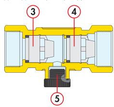
The double check valve may be used, where permitted by current local legislation, as an alternative to the backflow preventer, whenever the water distribution mains has low inlet pressure.
